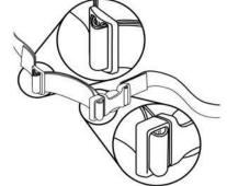
To remove the Adjustable Tension Back Upholstery, release the buckles on the straps.
