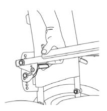
To flip up the locking Armrests, release the arm lock by lifting the blue trigger underneath the armrest tube and lift up the armrest.
